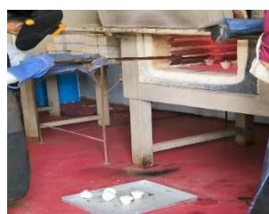
Gambar 7. Proses Pengujian Kadar Abu Briket
