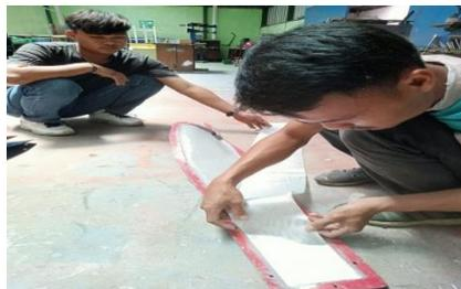
Gambar 6. Pemotongan Fiberglass
