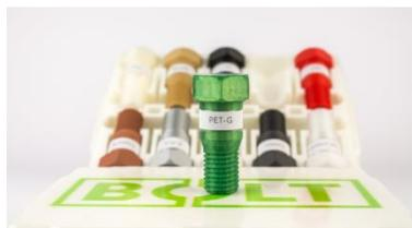
Gambar 17. Hasil Cetak Filamen Material PETG (Sumber: Leapfrog, 2020)
