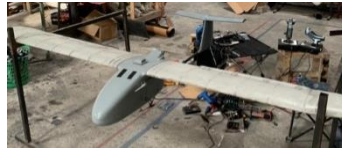
Gambar 6. Hasil Finishing Assembly Part UAV Skywalker 1900
