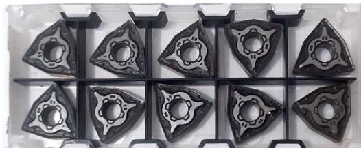
Gambar 3. Mata potong insert carbide merk WNMG
