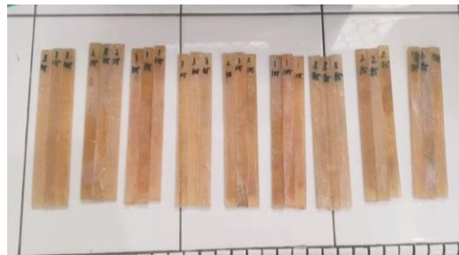
Gambar 4. Sampel Uji Tarik
