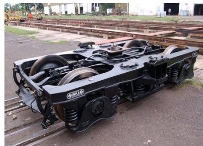
Figure 2. Bogie Structure Applied in Current Passenger Coaches [8]
