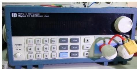
Gambar 3. Maynuo DC Electronic Load
