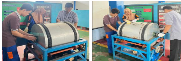
Gambar 3. Proses Assembly Mesin Pengering Gabah
