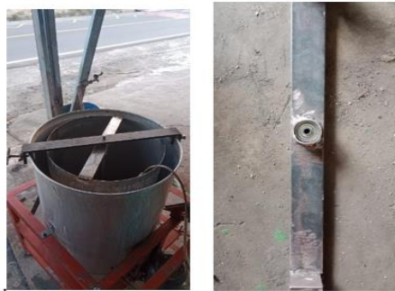
Gambar 7. Penambahan Bearing Penopang Poros Mesin
